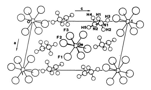
Fig. I. A view of the unit cell of  $(N_2H_5)_2GeF_6$  along [010] direction
